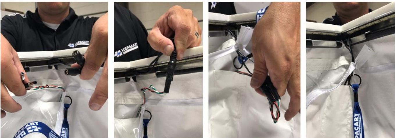
Figure 1.5: CURTAIN EXTENSION WIRES
