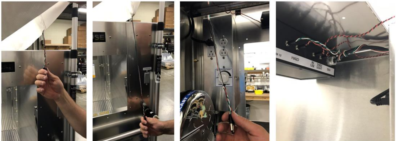
Figure 1.7: CURTAIN WIRES BOTTOM
