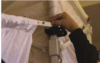
Spread the cuff and load the support poles
