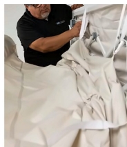
Secure the support straps to the upper truss
