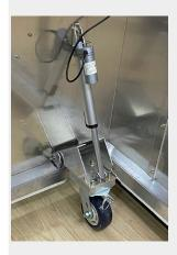
Removable casters and actuators to provide access to the corners.
