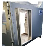
Exterior View: Open Wall Access Door w/ Foam Protected Flange.
